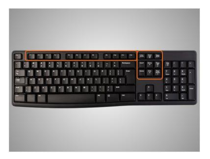
At the top of the keyboard are the function keys and special keys, which have specific uses.
