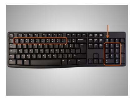
The number keys are located in two places on the keyboard. They are in the main section above the letters, and on larger keyboards in a number pad on the right side. This area of keys can either be arrow keys or number keys depending on whether the number lock key is on or off.
