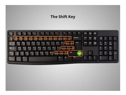
The Shift Key – This key is used for either capitalizing a letter or to access the symbols above the number keys and punctuation keys. When you hold down the shift key, either the capital letter is typed, or you are typing the character that appears on the top left of the key.
