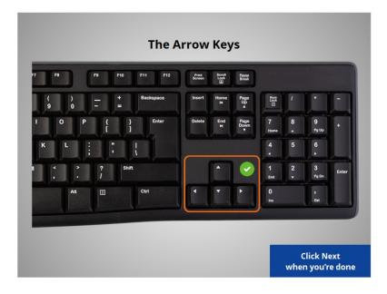
Arrow Keys – These are navigational keys that can help you go up, down, left and right when you are working on a document or when you want to scroll up and down a webpage.
