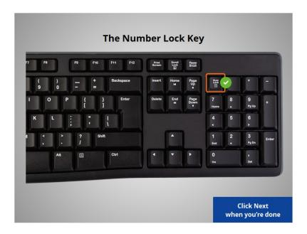
The Number Lock Key – Some keyboards have a number pad on the side, and if you turn on the Num Lock, the number pad will display numbers. If the Number Lock is not on, the number pad becomes a navigation pad like the arrow keys.
